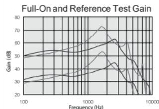
Measured according to ANSI S3.22-2014, IEC 60118-0:2015, JIS C 5512: 2015, 2cc coupler.
