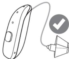
3. Check that the tulip dome is securely mounted by verifying that the collar completely covers the ribbed end of the receiver.
