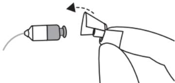
1. Remove the used dome by pulling it off the receiver and then discard it. This may require a bit of force.
