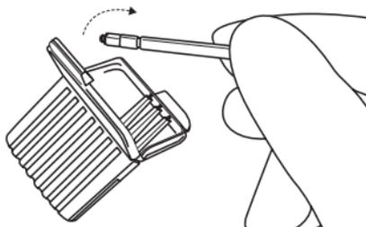
1. Remove the dome from the receiver.
