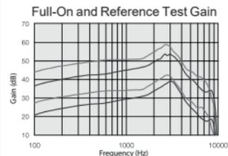
Measured according to ANSI S3.22-2014, IEC 60118-0:2015, JIS C 5512: 2015, 2cc coupler.
