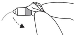
3. Check that the dome is securely mounted by carefully lifting the lower part of the dome and verifying that the collar completely covers the ribbed end of the receiver.
